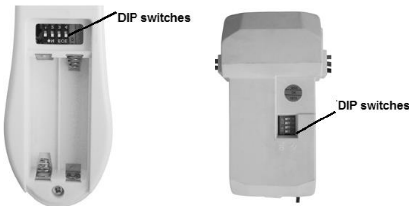
Fig. 11 Remote battery compartment
